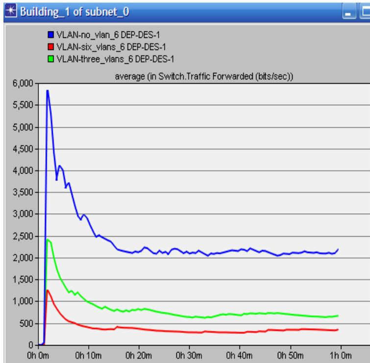
Figure 23: Average switch of building 1 traffic forwarded (bit/sec).
