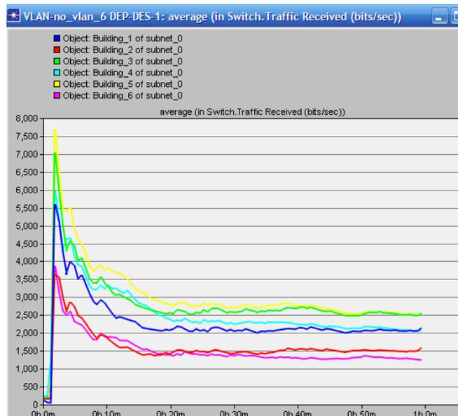
**Figure 19:** Traffic received in switch (bit/sec) for first scenario "NO\_vlan" with six departments.
