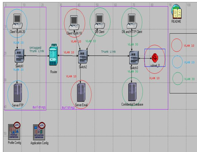
Figure 17: Scenario for "Inter-VLANs communication"
