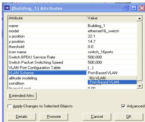
Figure 12: VLAN Scheme option Port-Based VLAN.
