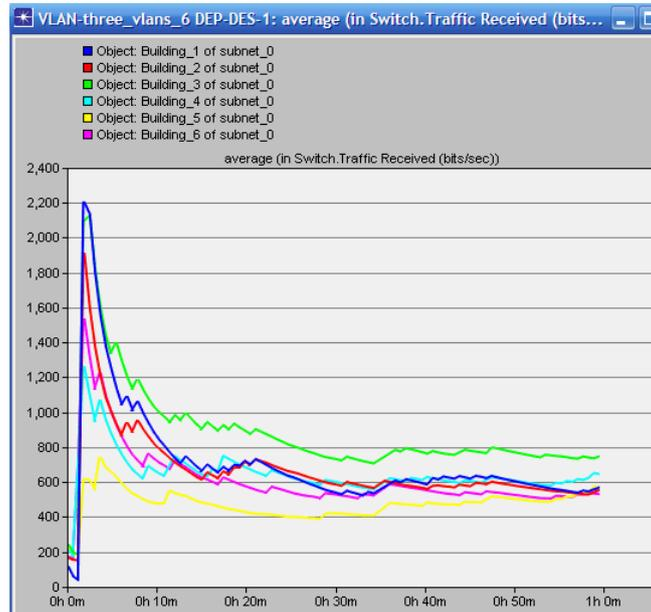
Figure 20: Traffic received in switch (bit/sec) for second scenario "3\_vlan" with six departments.
