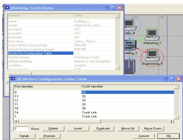
Figure 13: VLAN Scheme option Port-Based VLAN
