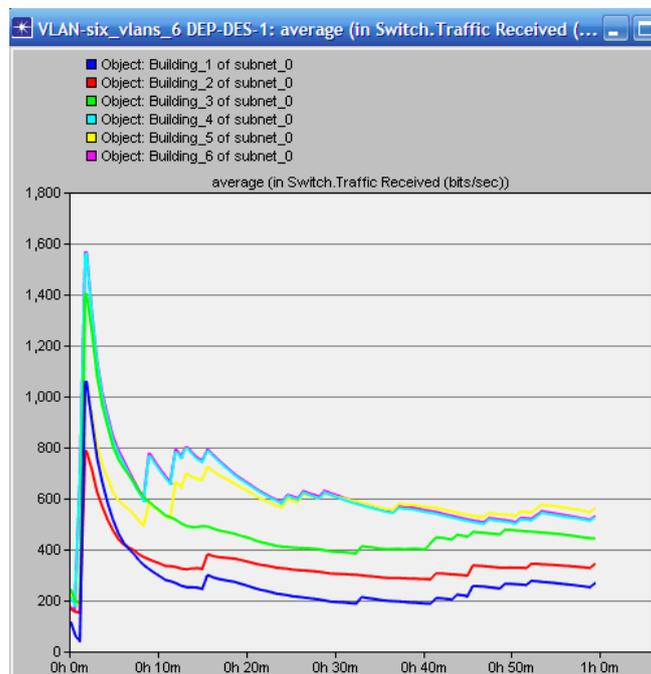
Figure 21: Traffic received in switch (bit/sec) for second scenario "6\_vlan" with six departments.
