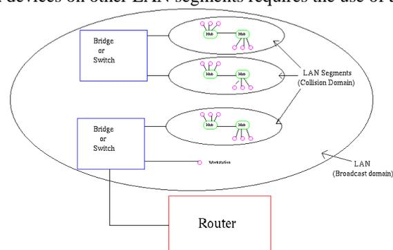
Figure 1: Physical view of a LAN.
